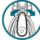
When storing, wrap cord around cord hooks. For quick cord access, rotate upper hook down and remove cord.
